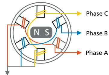
Figure - Representation of typical PM synchronous machine
